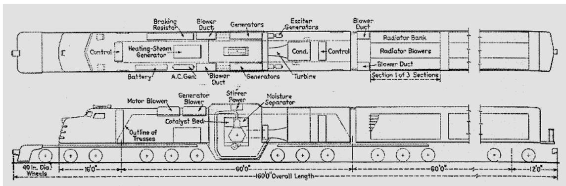
The engine section and its tender, which would have carried huge radiators for cooling the turbine steam, would have measured 160 feet in length; raising further questions about its ability to maneuver curved or steep sections of existing track.
