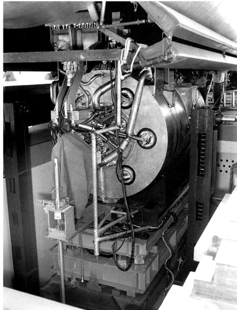
The aircraft's nose section was fitted with a unique cockpit assembly that encapsulated and shielded the crew whenever the reactor was started up in flight. This addition included twelve tons of shielding material and leaded glass windows ten-twelve inches thick. The following photo shows the assembly just prior to installation in the test aircraft.
