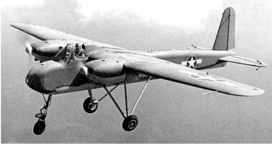
The TDN-1 had a wingspan of 48 feet. Two-220 HP Lycoming piston engines provided a maximum speed of 145 MPH. Ungainly, it had a tricycle landing gear to facilitate carrying a bomb or torpedo beneath its belly. It also had a removable cockpit so that it could be flown from the factory to operational air bases.
