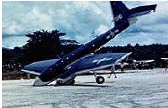
Not knowing that the 2,000-pound bomb slung beneath the drone had not yet been armed, people standing alongside the runway scattered frantically. Other than a smashed nose wheel assembly and two broken propellers, the only other damage was to the unit's pride.
