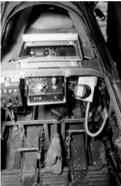
Because of the low priority given to Project Option, the designers of those controls had to improvise. Clearly visible on the panel in the center of the photo on the left is a joy stick...and an old-fashioned telephone rotary dial.
