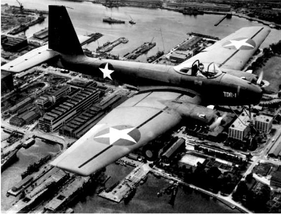
Initial flights were conducted in the latter half of 1943. Before the guidance system was tried, several of the aircraft were put through their paces by test pilots perched in TDR-1 temporary cockpits that had minimal controls and instruments. Nevertheless, one test pilot enthusiastically noted: *“It was exceptionally stable. You could do maneuvers in it that would stall out most conventional airplanes.”*
