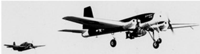
Once airborne and given control of the drone, a TBM-1C pilot would guide a TDR-1 to the vicinity of the tall, slender structure. Control of the drone was then handed off to another pilot, seated in the rear of the mother ship. Under a black cloth hood, he would peer at a six-diameter TV screen, shown below on the right side of his rudimentary control panel when zeroing in on a target.
